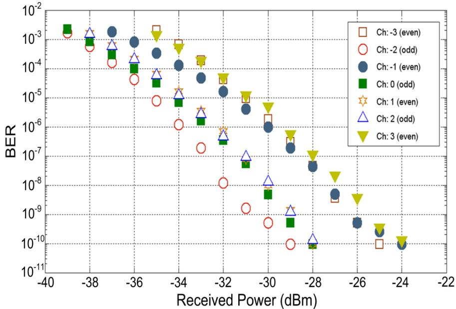
Figure 5 : Measured BER against received optical power for the 74.648Gb/s CoWDM system when the phase was optimized.
