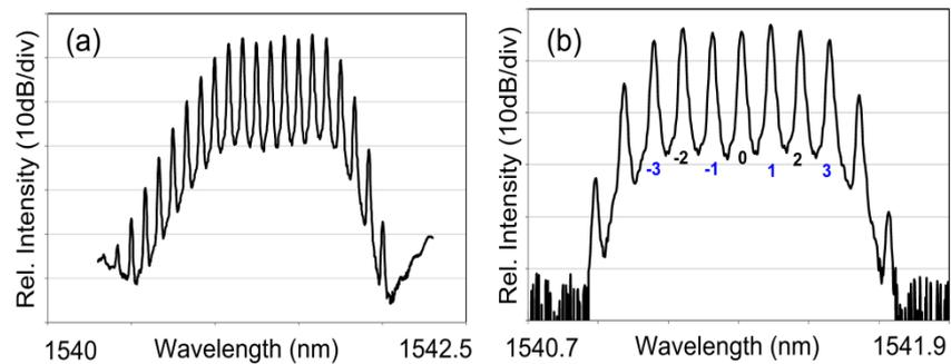
Figure 1 : Optical spectra (a) output comb from PP-OWCS (b) 7 filtered lines from PP-OWCS
