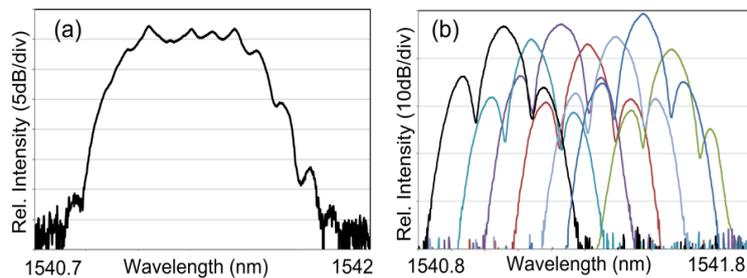
**Figure 3 : Optical spectra of (a) 74.648Gb/s CoWDM signal at the Tx and (b) 7 individual filtered DPSK sub-channels each at 10.664Gb/s at the Rx.**
