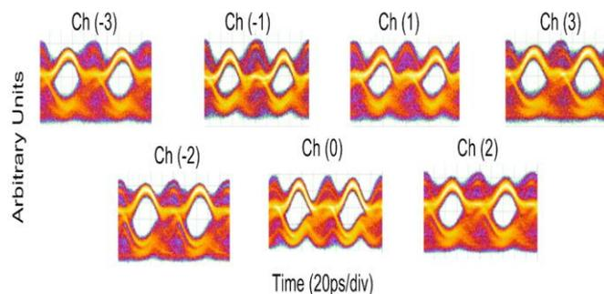
**Figure 4: Eye diagrams of the 7 demodulated odd and even subcarriers.**
