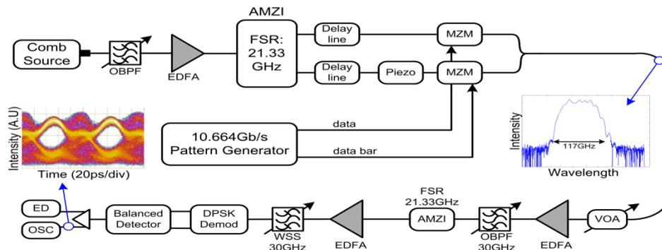
Figure 2 : Experimental configuration of the CoWDM system employing a gain switched DM laser transmitter
