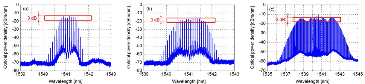
**Fig. 1** Optical comb produced by gain switched DM-LD.(a), and its further expansion with use of phase modulator (b) and nonlinearities of optical fiber (c). The optical spectra recorded with a high resolution optical spectrum analyzer.
